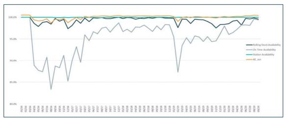
Figure 9-5 Availability Ratio Components and their relation with the Availability Factor until September 2020
