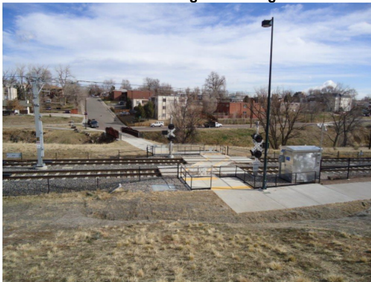
Figure 9 Pedestrian Crossing with Z Crossings
