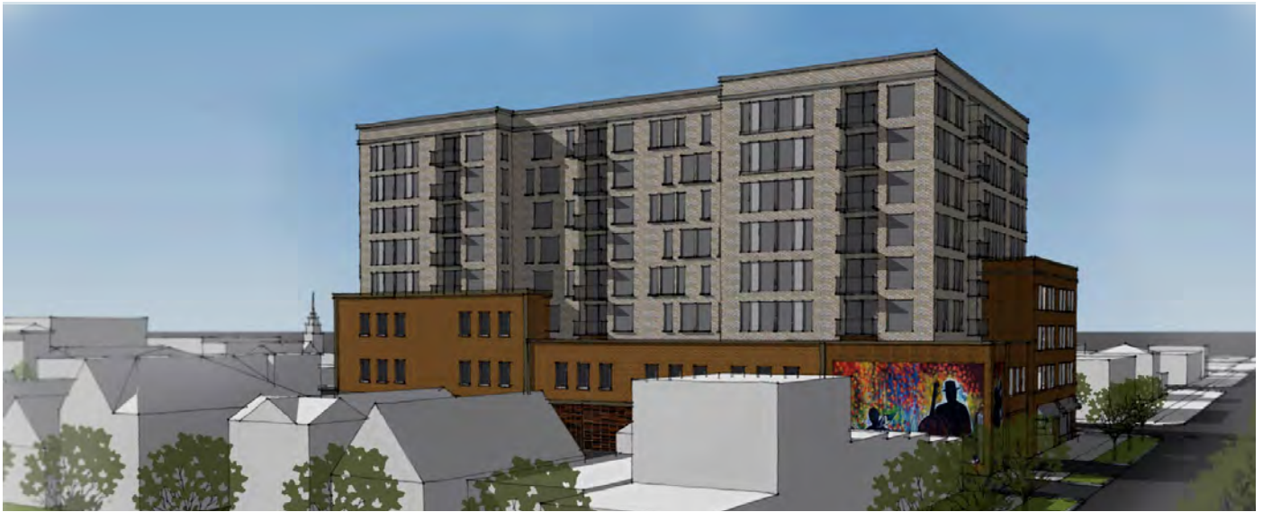
Large infill massing adjacent to residential context, showing a fully articulated facade to reduce the appearance of scale and Upper Story Setbacks to vary the massing without creating excessive modulation.
