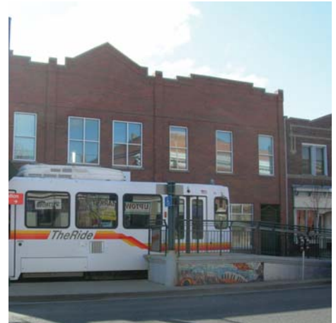
If streetcar replaced light rail on Welton, the dedicated right of way and high block platforms could be removed and used to enhance the pedestrian realm.
