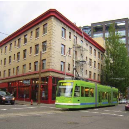
Streetcars operate in mixed traffic with other vehicles and are smaller and more nimble than light rail.
