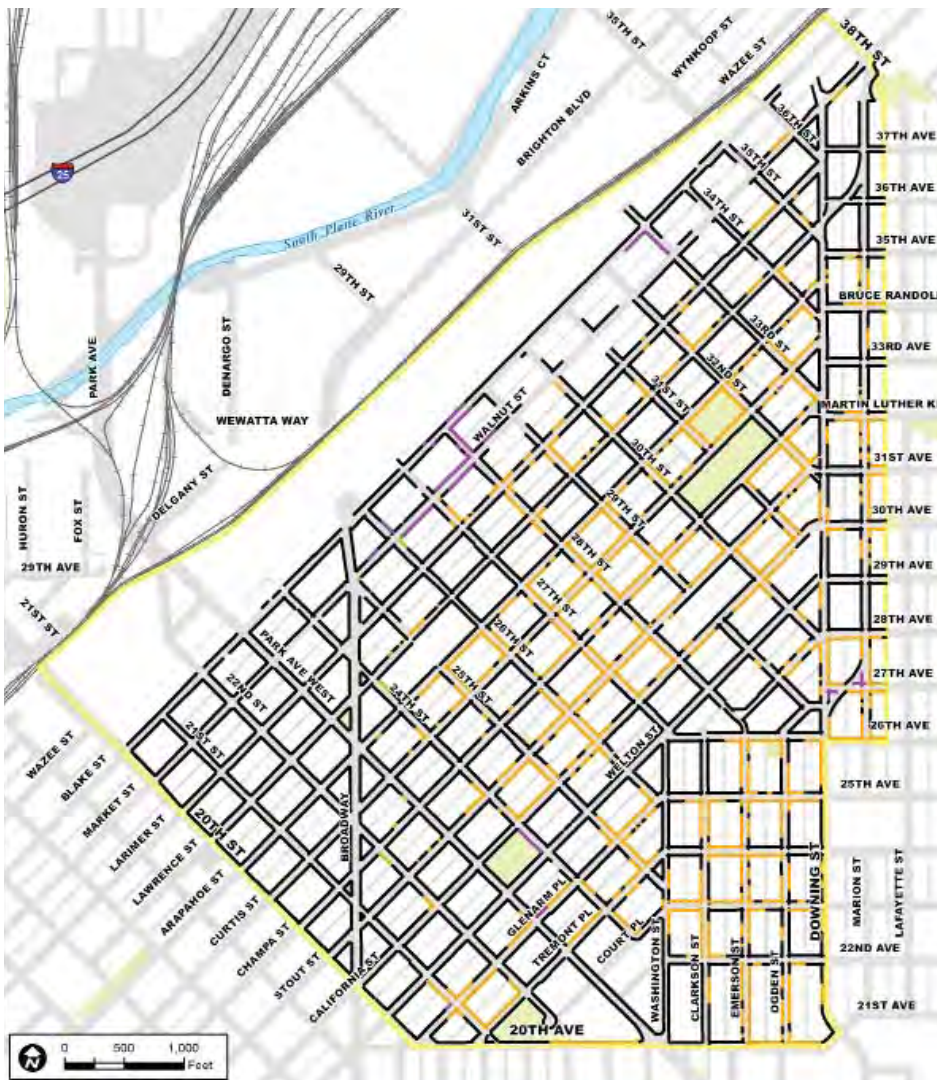
Existing Sidewalk Surface Material Map
