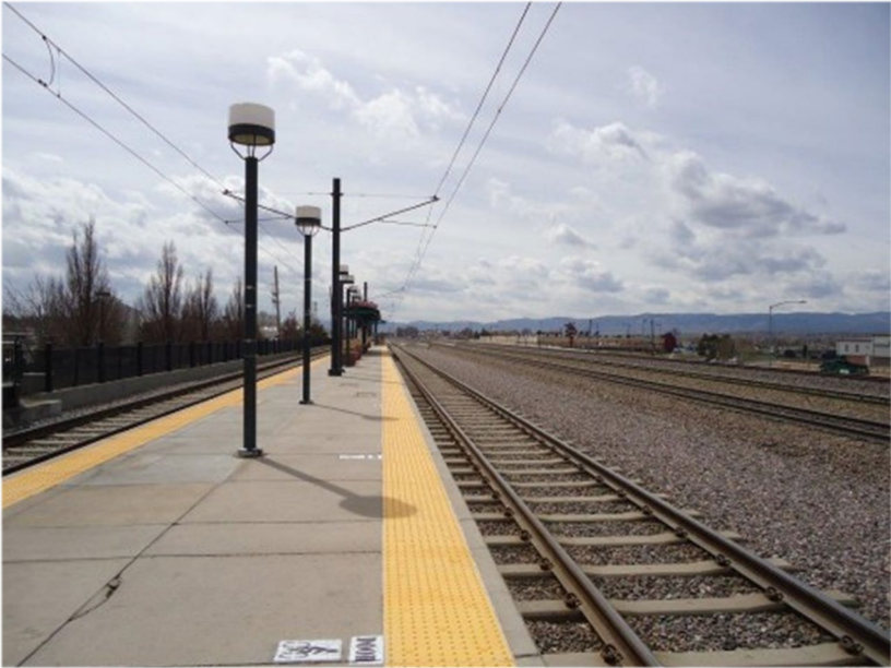
FIGURE 2 - EXCLUSIVE ALIGNMENT ADJACENT TO FREIGHT RAIL CORRIDOR
