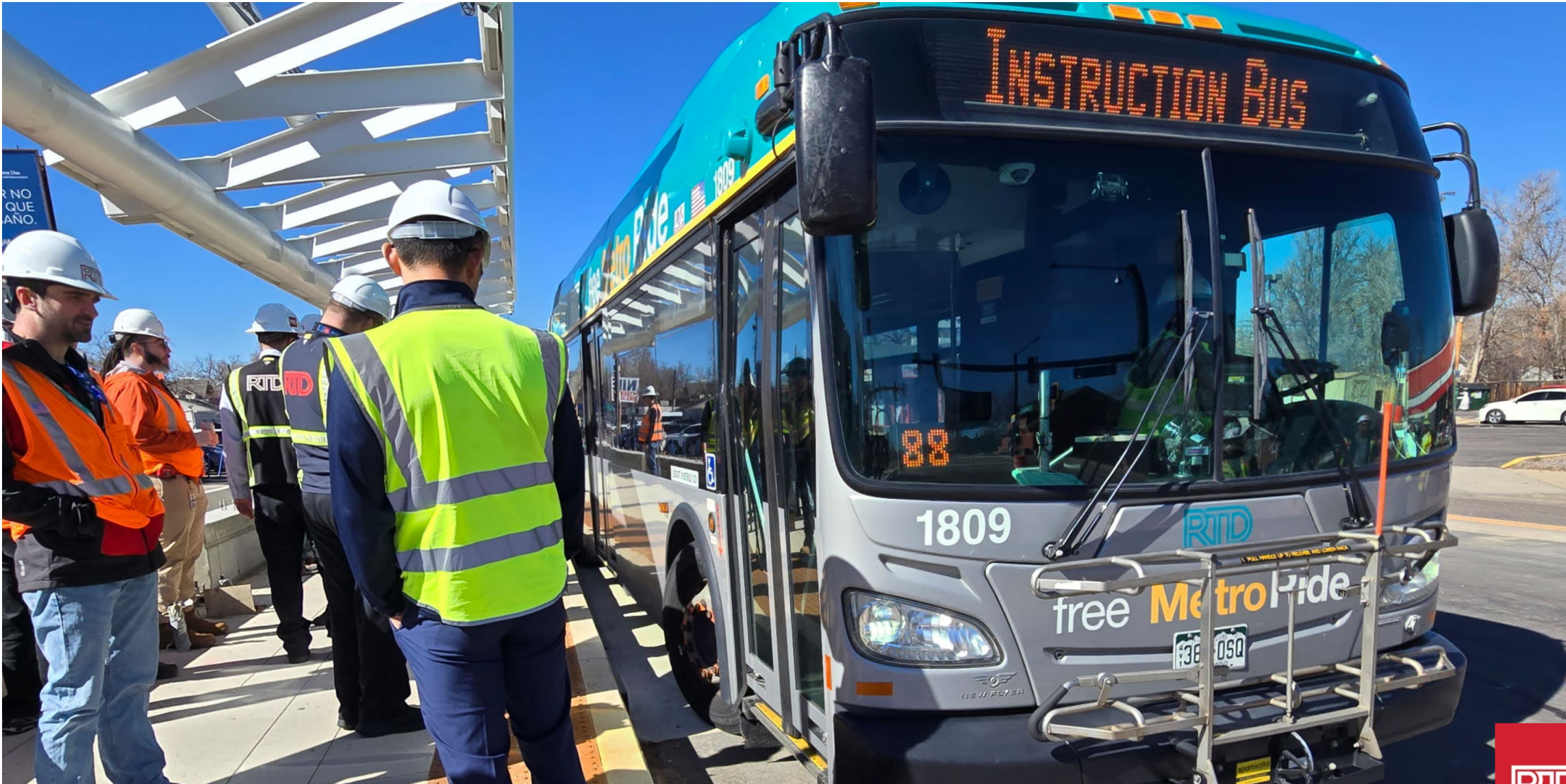
East Colfax Bus Rapid Transit (BRT) level boarding testing
