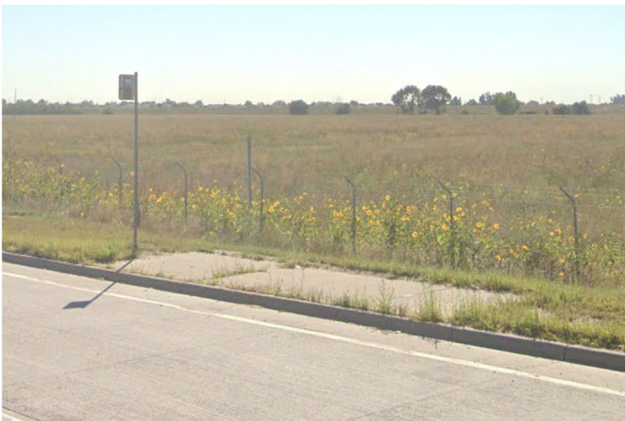
Figure 3-29: Field-Verified ADA Limitation for Presence of Accessible Path of Travel at 120th Ave & Brighton Rd in Commerce City (33033)
