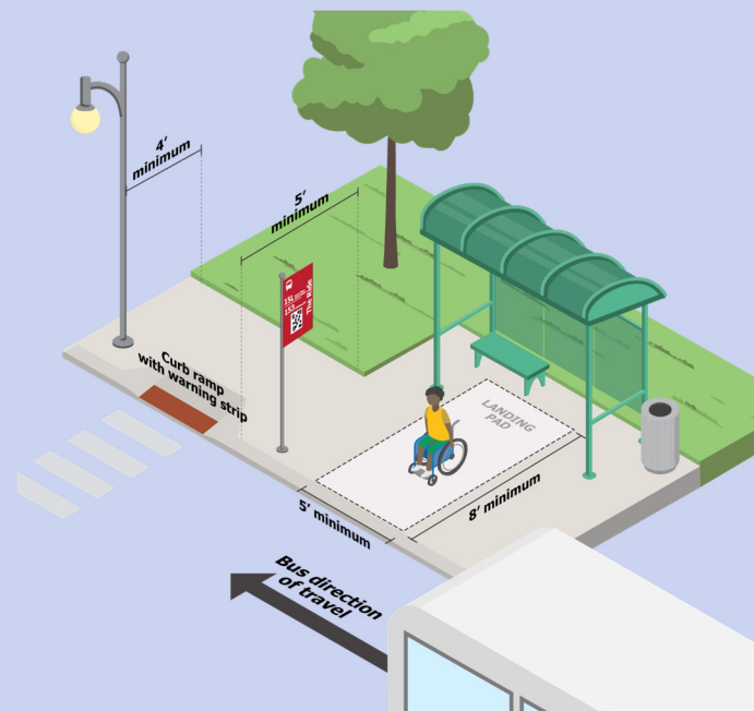
Figure 3-2: Stop Accessibility Dimensions
